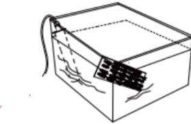
If no ultrasonic cleaner, try to use an ultrasonic rod to clean for 2-3min.
