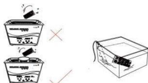
**6.** It is recommended to put the prints in a container with alcohol fully cover while using ultrasonic machine which is safer. If there is no ultrasonic cleaner, try to use an ultrasonic rod.
