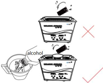
5. Soak the prints in alcohol in container, clean for 1-2min by ultrasonic machine.
