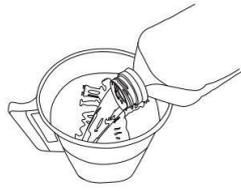
6.Place the work piece into a container with alcohol, the alcohol should fully cover for 5-10mins.
