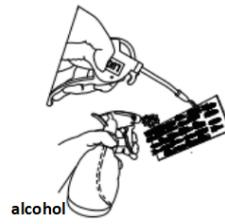
**3.** Spray alcohol again, dry it with air gun, repeat a few times till there's no resin on surface.
