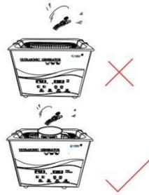
7.Put the container into ultrasonic machine, clean for 1-2 mins.
