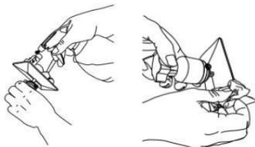
**2.** Spray Isopropanol (alcohol > 95%) to clean away residue resin that on the prints and wipe off the resin with tissue from the platform.
