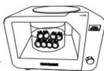
**9.** Suggest to do post curing in water, curing time depends on the light power of the curing box and thickness of the prints.
