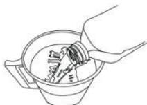
**5.** Place the work piece into a container with alcohol, the alcohol should fully cover it.
