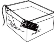
If no ultrasonic cleaner, try to use an ultrasonic rod to clean for 2-3min.
