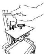
**1.** Remove the printing platform from the printer.
