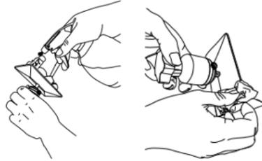
2. Spray isopropanol (alcohol > 95%) to clean away residue resin on the prints, wipe off the resin with tissue on the platform.
