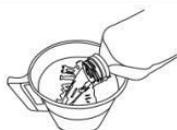
**9.** After step **8**, prepare a container with fresh alcohol, soak in IPA for 30mins.
