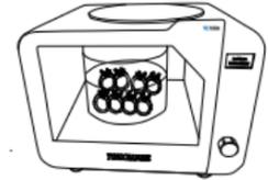
7. Suggest post curing in water, curing time 30-60s depends on the light power of the curing box (curing both sides).
