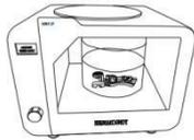
10. Suggest to do post curing in water, curing time depends on the light power of the curing box, or blower.
