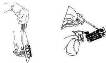
**4.** Carefully take off the prints from platform with scraper. Spray alcohol again then dry it with air gun, repeat a few times till there's no resin on surface.
