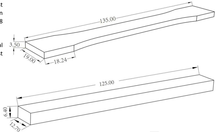
specimen ASTM D790
